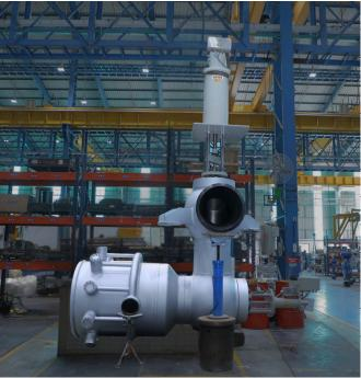
A major Eastern Indian power plant required a reliable LP bypass valve solution for uninterrupted power supply and optimized efficiency. The challenge demanded a valve handling temperatures up to 601°C, crafted from ASTM A182 F91 forging.
