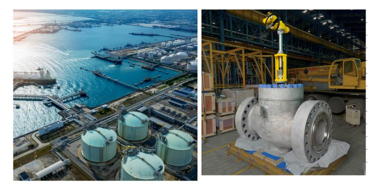
Size becomes a testament to engineering prowess when Saudi Arabia's state oil company needed a 30" Globe valve - the largest we've manufactured. The project, aimed at enhancing crude oil processing capabilities, required a valve design compliant with ASME BPVC Section VIII standards.
