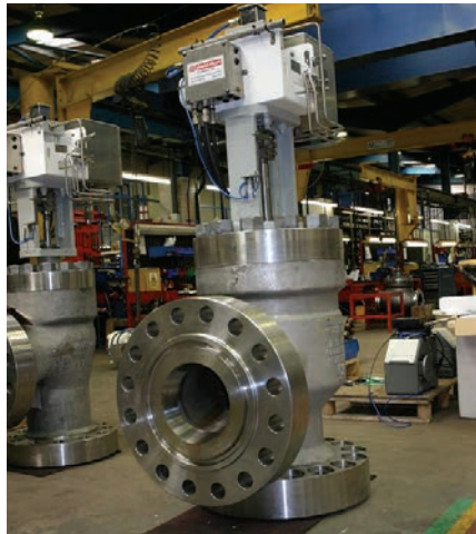
12" ANSI 1500 choke C/W electro-hydraulic actuator
