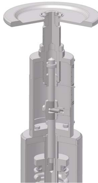
Fig. 2 top mounted handwheel/ jacking screw
