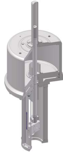
Fig. 11 'D' series Pneumatic Double Acting Actuator
