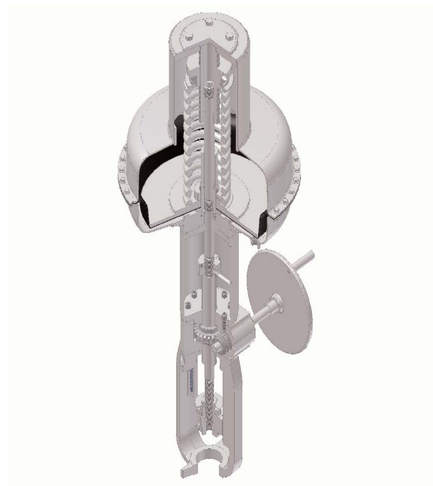
Fig. 3. Side mounted Handwheel Unit
